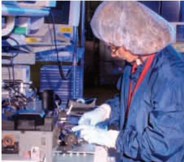
FIGURE 1. At the JDS Uniphase clean room in Bloomfield, CT, an assembler attaches optical fibers to the internal optical components of a modulator for use in telecom amplification. Such components will become RoHS-compliant according to the company.
